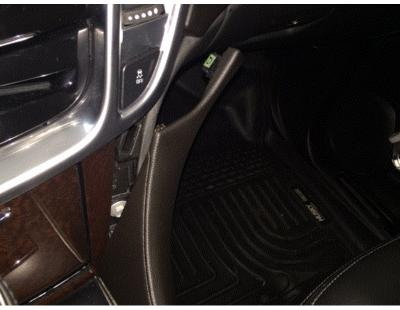
2. Pry the upper portion of the U shaped (wood grained) trim the surrounds the lower storage unit. Pry the top and middle of each arm in the U then pull the piece upward.
