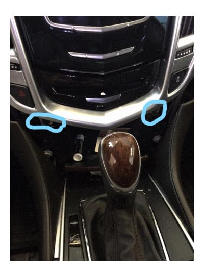
4. Pry the trim piece that is directly above the touch screen straight towards the back of the vehicle. Pry one side, center then other side.
